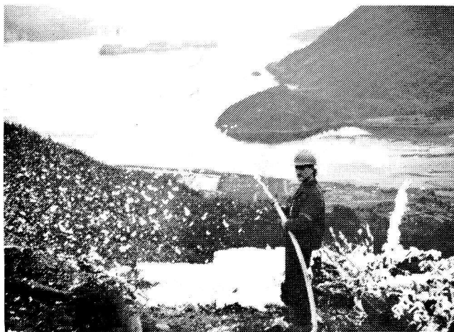
Figure 14. Dynamic foam flow at 820-ft vertical elevation above the pump.
