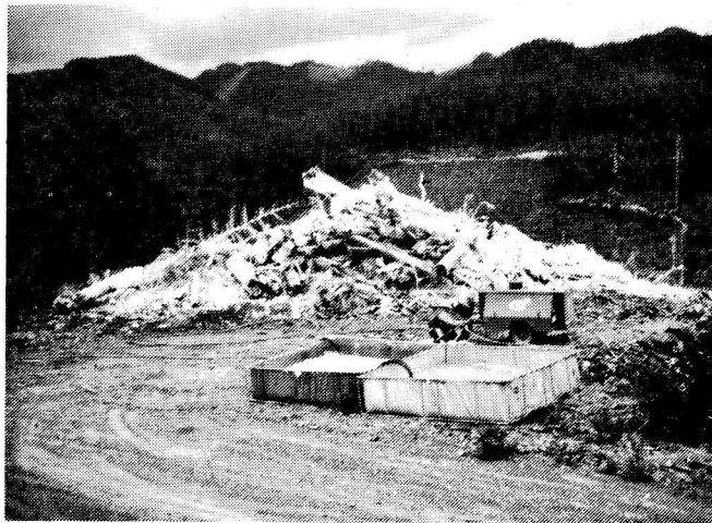
Figure 2. CAFS adds air from trailer compressor to foam solution pumped from portable tanks in order to foam the log deck.
