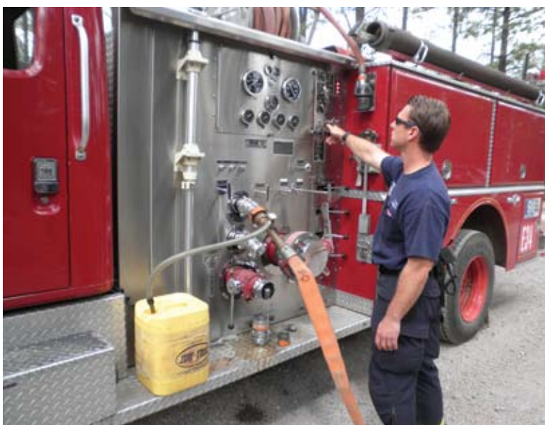
A firefighter operates a foam eductor. Remember: Eductors can be great tools, but they must be set up and operated properly to be effective.
